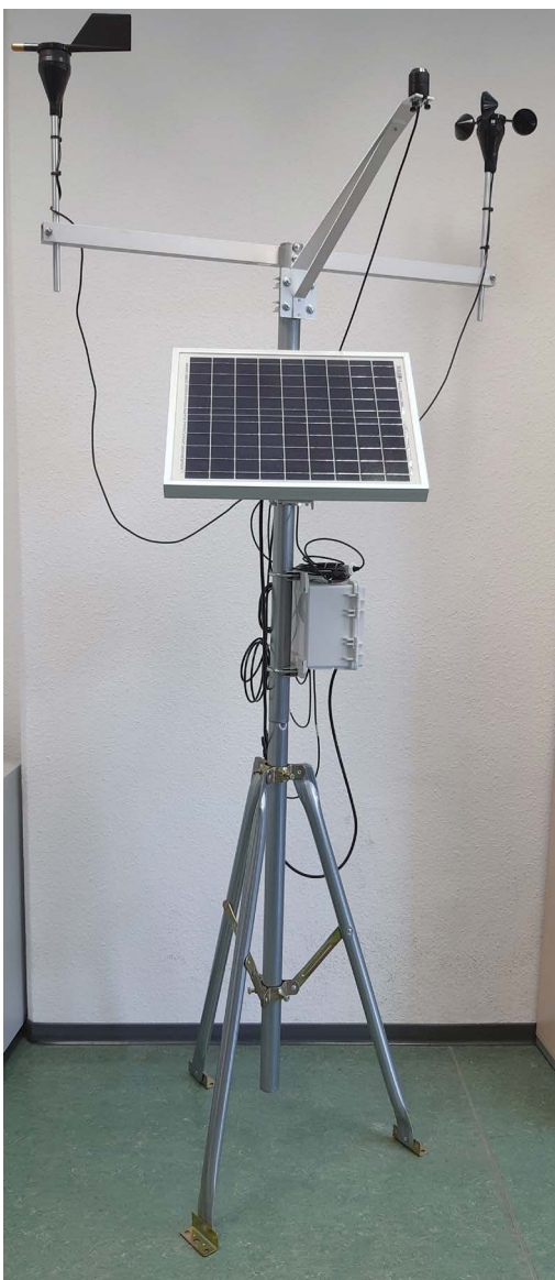
Abb. 17 Versuch Wetterstation, © Abel
